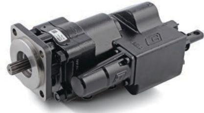
Parker's Commercial brand SG102 Series dump pump is designed to fit where space is limited, but greater flow is still a necessity. The SG102 dump pump utilizes the valve body of the larger frame size C Series dump pump, providing large dump pump flow characteristics for a faster dump cycle time, yielding greater work cycle efficiency.
